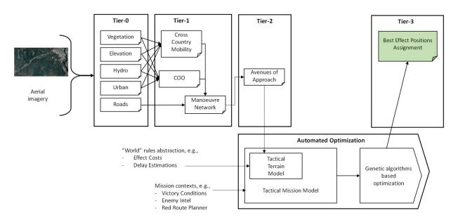
Figure 7: Overview of the products involved in the COSMOS prototype. The green Tier-3 TSO product was generated by the Automated Optimization process, in this case using a genetic algorithm.
