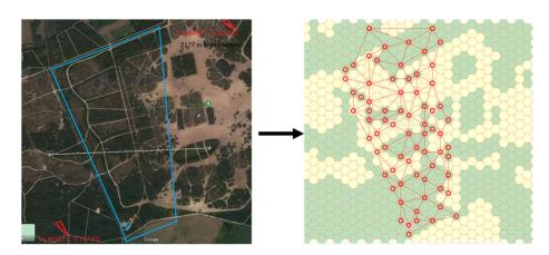
Figure 12: Transformation of the raw data to an abstracted Tactical Terrain Model using hexagons and a sparse manoeuvre graph.
